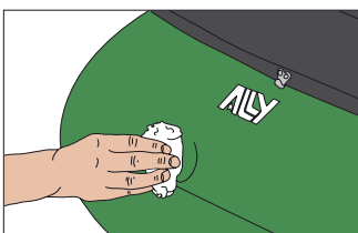
4. To enhance the bond, wash both the marked canoe skin bond area and the attach-loop bond area with acetone. A simple cotton cloth may be used.
